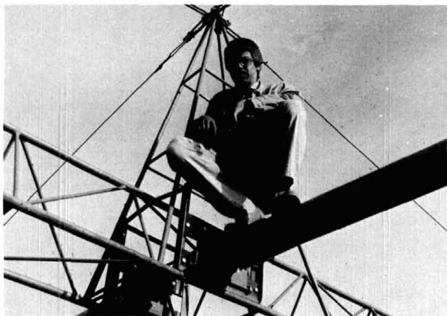
fig. 7. Peter, OH1RY, atop the driven element of his 80-meter Yagi. Center of element is 6 inches (15.24 cm) in diameter!
